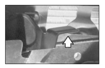
Then go to the front of the vehicle and lift up on the secondary hood release handle. The secondary hood release lever is located near the front center of the hood toward the driver's side.
